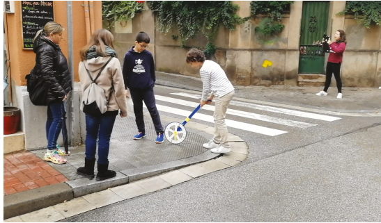
Figure 5. Fieldwork measuring the width of the sidewalk mounted by cars when turning.
