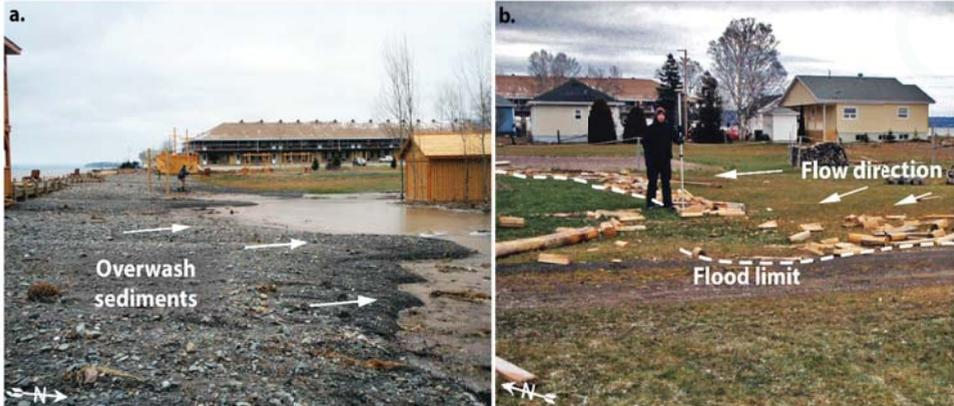
**Figure 3.** Field survey after the flood showing (a) flood generated overwash fan and (b) the debris line delineation. Limits were located using DGPS on the day following the storm event (Maria, 7 December 2010).
