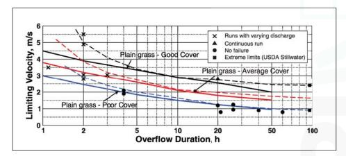
Figure 2. Erosion resistance of grass-lined spillways (after Whitehead et al. [12]).
