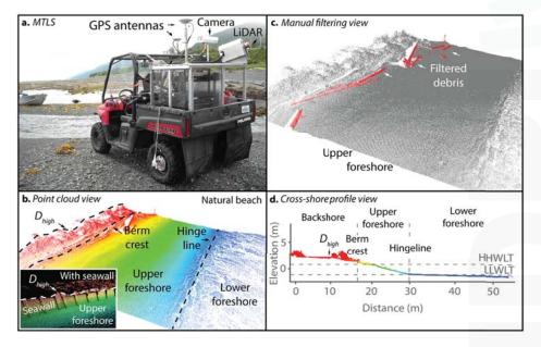
**Figure 4.** Mobile terrestrial LiDAR system (**a**) with point cloud and filtering view examples (**b**,**c**). Resulting data are used in cross-shore view to localize the first ridge on the natural beach or the coastal structure crest elevation ( $D_{high}$ ), the berm crest and the hinge line (**d**).
