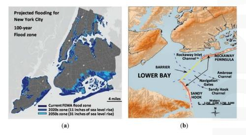
Figure 11. (a) NYC projected flooded areas for 100-year storm, SLR 79 cm by 2050 [23]. (b) Proposed surge barriers [24] and surge barrier with gates [24].
