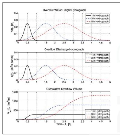
Figure 5. Idealized overflow hydrographs and cumulative overflow water volume.
