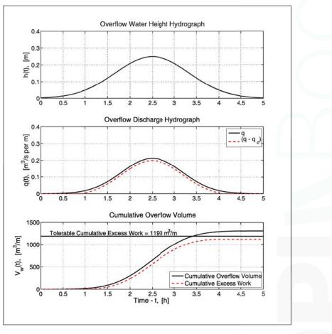
**Figure 6.** Example of cumulative excess work estimate for "good grass" ( $u_c = 1.8 \text{ m/s}$ ).
