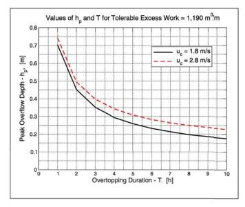
**Figure 8.** Equivalence pairs of peak overflow depth and overtopping duration that produce tolerable cumulative excess work of  $V_{ET}$  = 1190 m<sup>3</sup>/m.
