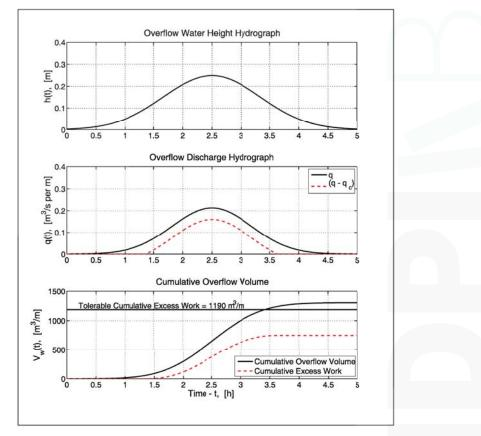
**Figure 7.** Example of cumulative excess work estimate for grass with  $u_c = 2.8$  m/s.
