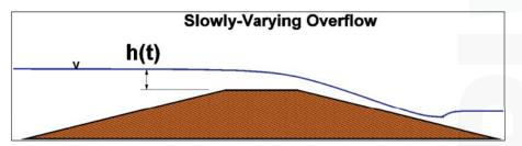
Figure 4. Slowly-varying overflow of a levee.
