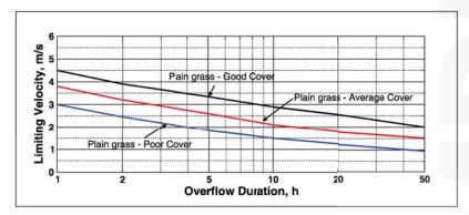
Figure 1. Limiting velocity versus overflow duration for grass (after Hewlett et al. [11]).
