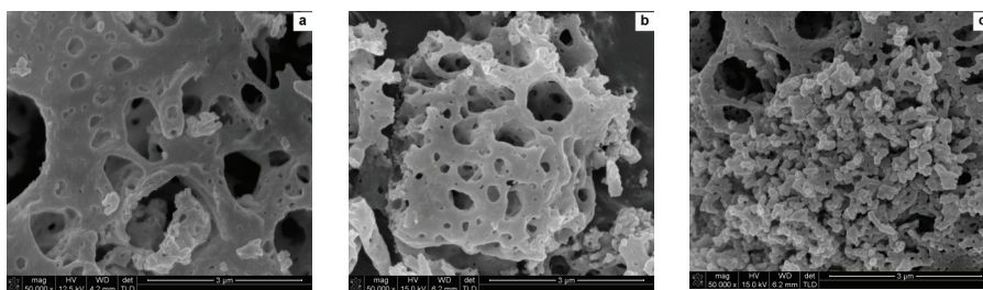
Figure 4. Micrographs of yttria nanopowder obtained by solution combustion synthesis (SCS) by the reaction of yttria nitrate with glycine: (a) not calcined, (b) calcined at a temperature of 800 °C, (c) calcined at a temperature of 1100 °C.
