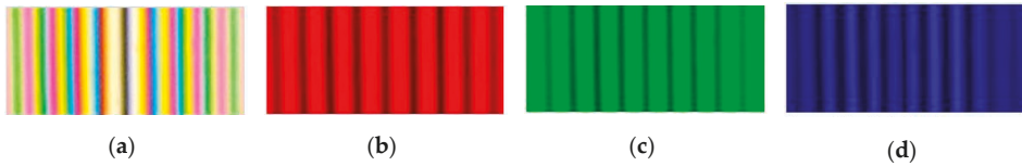
Figure 2. The interference pattern of white light and RGB light interference components. (a) White light interference pattern; (b) red light interference pattern; (c) green light interference pattern; (d) blue light interference pattern.
