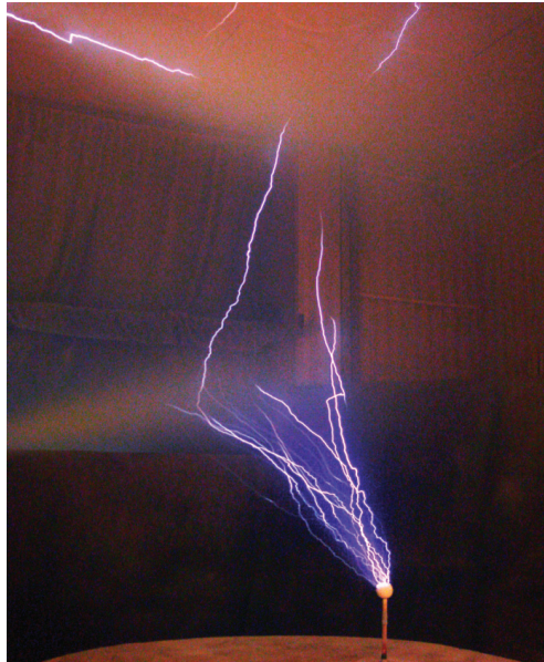
Figure 4. Characteristic picture of the discharge formation between the system of artificial thunderstorm cells of negative polarity and the ground.
