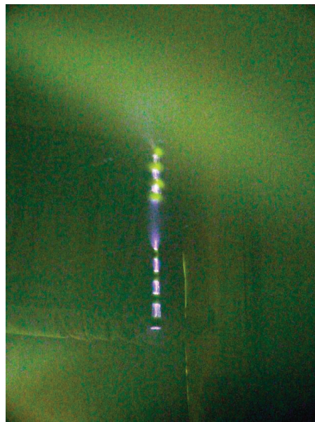
Figure 3. Characteristic picture of the discharge formation between positively and negatively charged artificial thunderstorm cells, using model hydrometeor groups.
