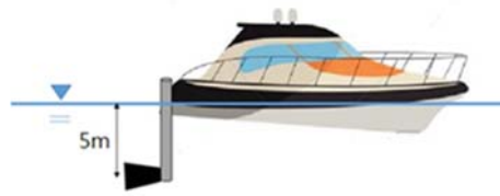
Figure 7. Schematic of the installation position of the projector.
