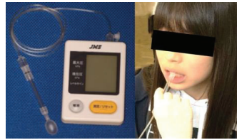
Figure 10. Tongue pressure force measurement. The tongue pressure force was measured using a TPM01 (JMS Co. Ltd., Hiroshima, Japan). The patient sat with the Frankfurt plane parallel to the clinic floor. The balloon was inserted into the mouth, and the patient was instructed to lightly bite down on the hard ring with the upper and lower central incisors, to secure the balloon to the anterior part of the palate.
