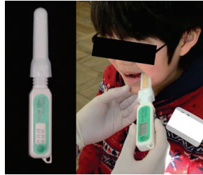
Figure 8. Occlusal force measurement. The occlusal force was measured using GM10 (Nagano Keiki Co. Ltd., Tokyo, Japan). The subjects were seated in the Frankfurt horizontal plane parallel to the floor. The sensor was placed in the maxillary first molar, and the occlusal force was measured.
