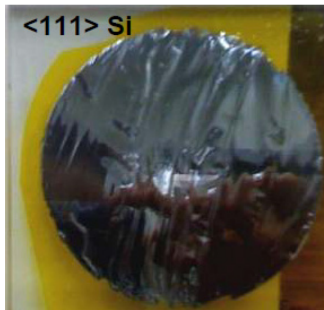
Figure 5. Spalling of Si(111), wafer <111> from the ingot of a diameter of 100 mm.
