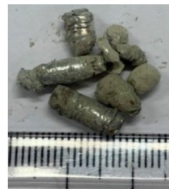
Figure 5. Photographs of the back-extruded aluminum during processing when the offset between the hole and the processing material is low during processing using 4- and 6-mm hole sizes.
