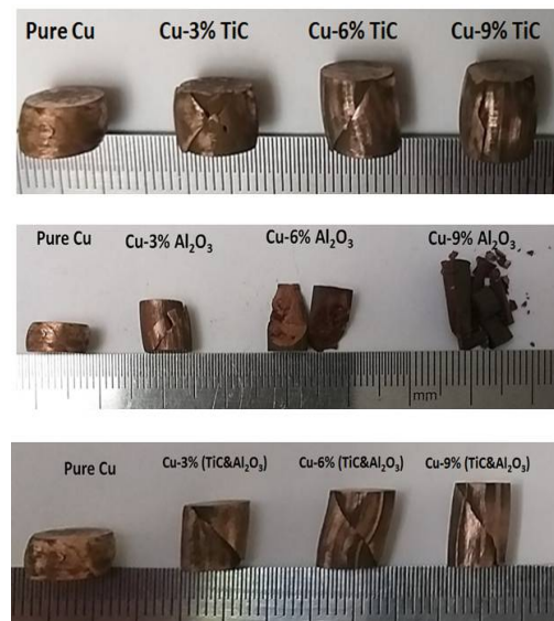
Figure 10. Compressed test samples for pure Cu and Cu matrix nanocomposites.
