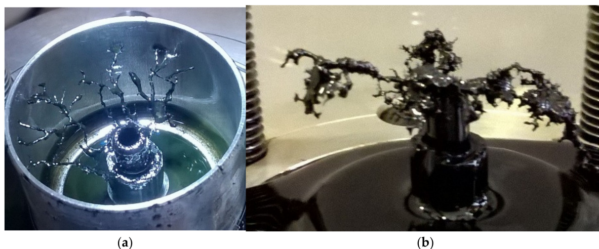
Figure 9. Photographs of tree-like structures formed: in microwave discharge in liquid engine oil (a); and in liquid residues of heavy petroleum feedstock (b).
