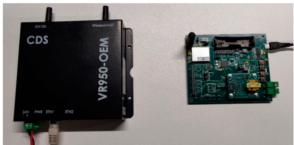
Figure 5. The ISA100.11a certified devices employed in the experimental setup: CDS VR950 gateway (left) and CDS VS210 field device (right).
