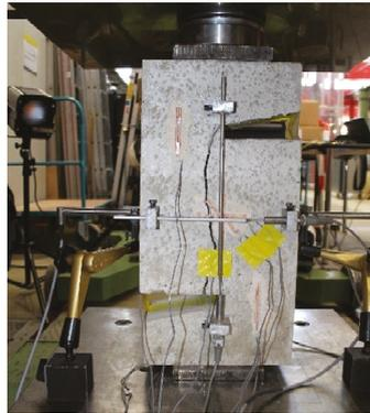
Figure 11. Typical failure of the monolithic specimen.
