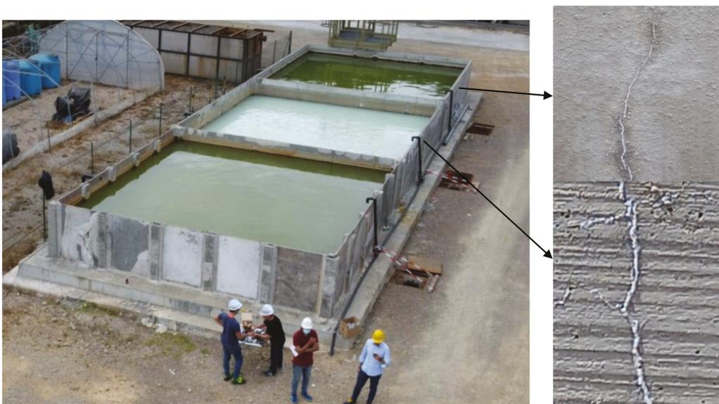
**Figure 20.** Evidence of crack sealing as monitored during a water filling test of the pilot on 14 May 2021.
