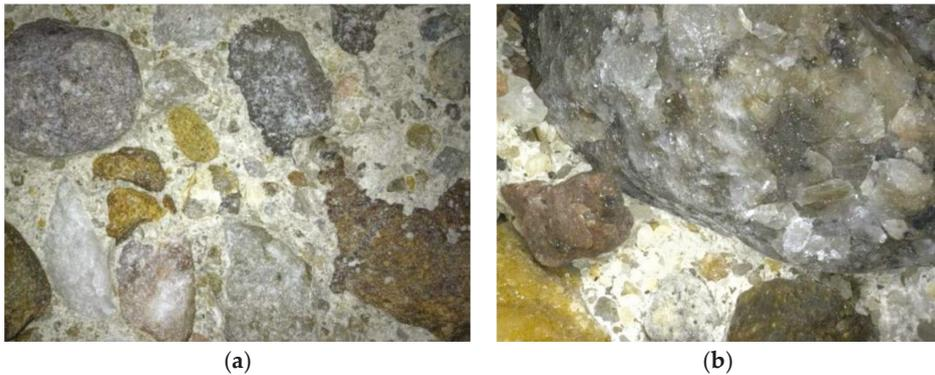
**Figure 7.** Detailed imaging of a sandblasted interface (a) and a water-jetted interface (b).
