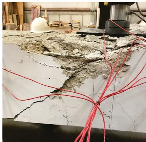
Figure 11. (a) Load–deflection relationship and (b) failure mode when loaded at midspan.
