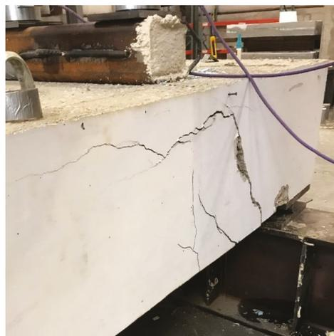
Figure 13. Failure mode when loaded at  $1.25d$ .
