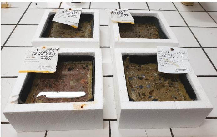
Figure 8. Samples exposed to freeze–thaw cycles.
