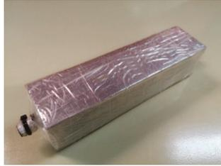
**Figure 2.** Sample for measurement of autogenous shrinkage.
