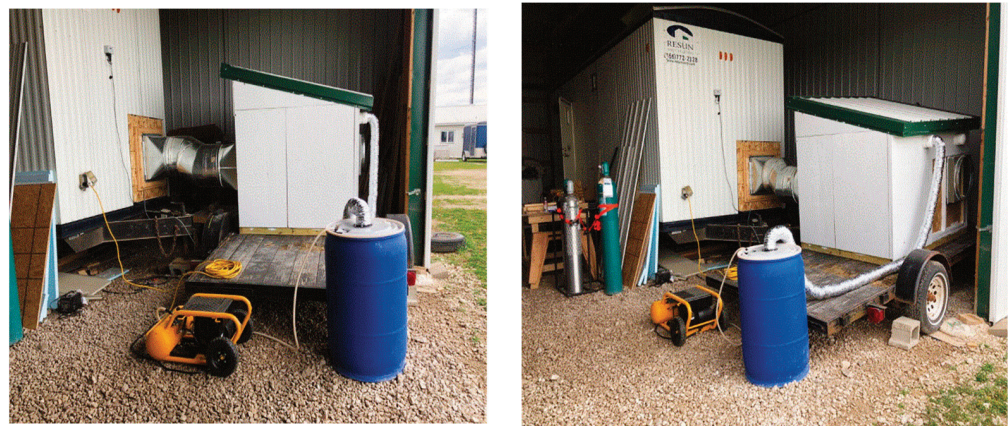
Figure A1. Picture of UV mobile laboratory (back) and filter house mounted on a trailer (front) with manure drum and gaseous emission generation system.
