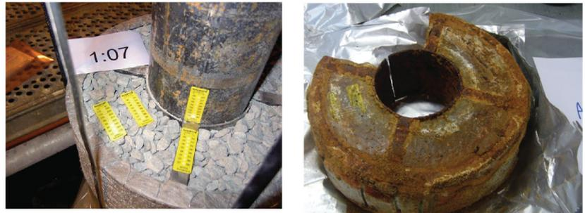
**Figure 3.** Example of caged pellets before installation (left) and after dismantling (right) [29].
