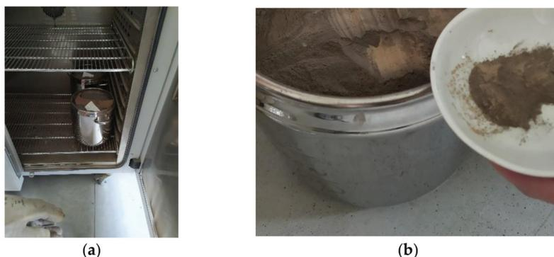
**Figure 1.** (a) Thermal loading of bentonite powder in open vessels, and (b) visible colour change from light brown to dark brown at the powder surface observed during sampling.
