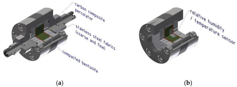
**Figure 2.** Experimental cell set-up for measuring (a) saturated hydraulic conductivity and (b) water retention curves.
