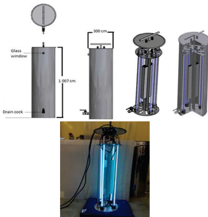
Figure 2. The portable photolytic cell. From left to right: external aspect and dimensions of the system case, scheme of the UV lamps support, the support inside the case system. Below, a photo of the completed lamps' support.
