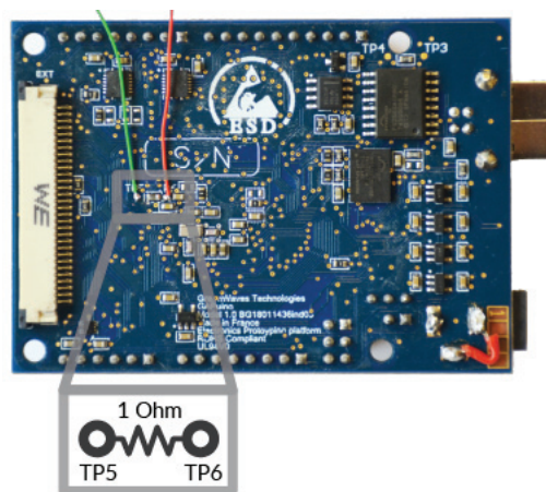
Figure A1. Measurement setup for power consumption showing a R = 1 \Omega shunt resistor at the bottom of the of the GAPuino evaluation [23] board with two measurement points (TP5 and TP6).
