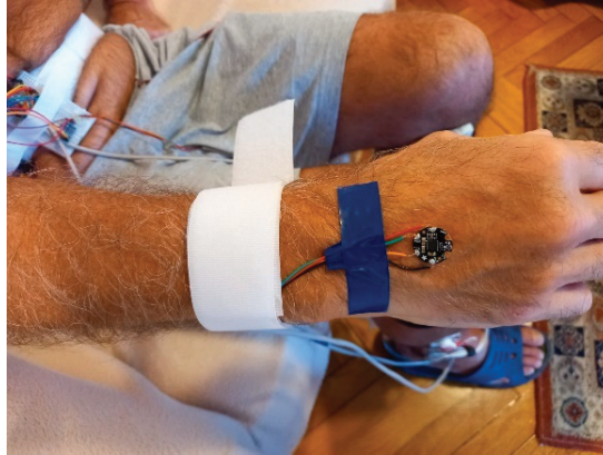
Figure 6. Illustration of the attachment of the LSM9DS0 accelerometer to the user's right wrist, for arm balance tracking during the gait cycle.
