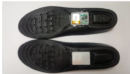
Figure 2. Sensor attachments to the insoles.
