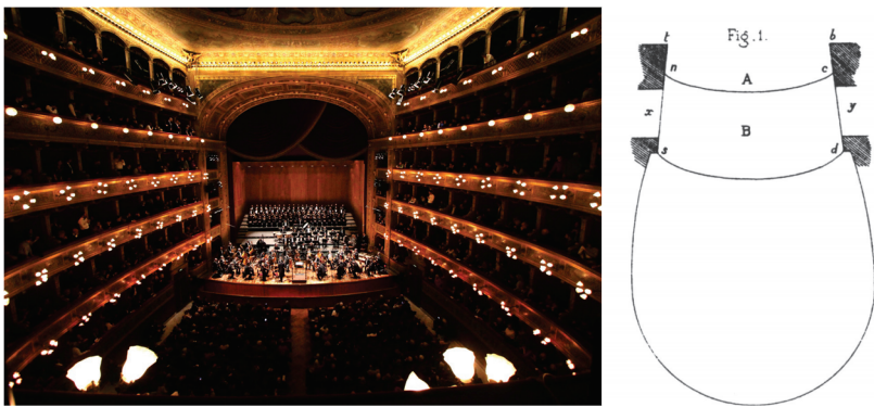
Figure 6. On the left: Proscenium arch of Massimo Theatre in Palermo; Reproduced with permission from Teatro Massimo, Copyright Franco Lannino, 2020. On the right: plan of Massimo theatre in Palermo A: proscenium, B: orchestra; btsd : proscenium arch; x, y : stage boxes.
