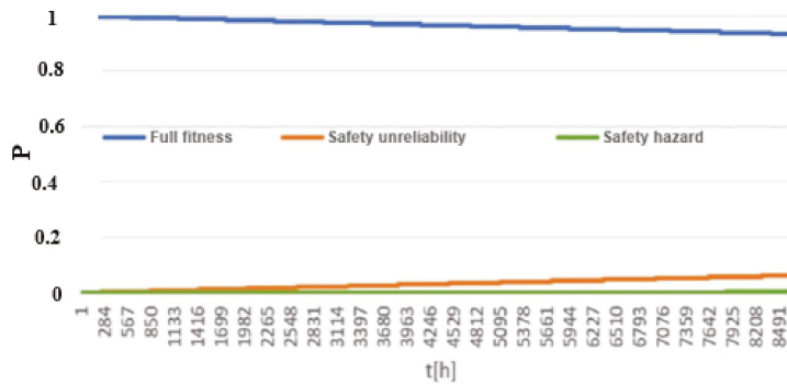
Figure 11. Probability functions for a system staying in one of the three primary states.
