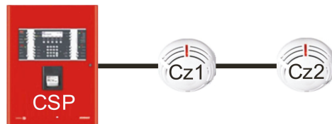
Figure 7. Simplified FAS diagram. CSP (FACU)—fire alarm control unit, Cz1, Cz2—detectors within the system detection line.
