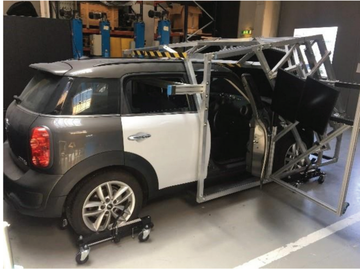
Figure 2. Automated driving simulator of Graz (ADSG). To cancel the external noise and adjust the indoor temperature, ADSG is separated from its surrounding area using an insulating housing cube.
