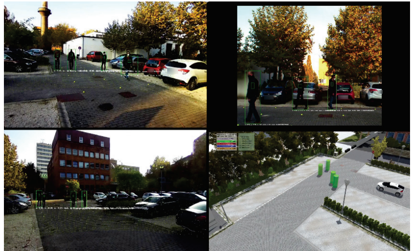
Figure 17. Top-left image: objects sensed by the infrastructure-1; Bottom-left image: objects sensed by the infrastructure-2; Top-right image: objects sensed by the vehicle; Bottom-right image: Real-time digital twin generated by the central system.
