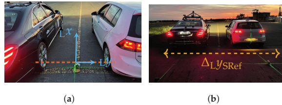
Figure 3. Dual-car calibration setup. Super-reference is provided by perpendicular cross line laser lines. (a) Zero longitudinal offset (i.e., \Delta_L x_{SRef} = 0 ) between the vehicles is verified by cross line laser through center of rear axles. (b) Lateral offset is obtained by measuring the distance between cross line laser lines focusing along the vehicle’s middle axis.
