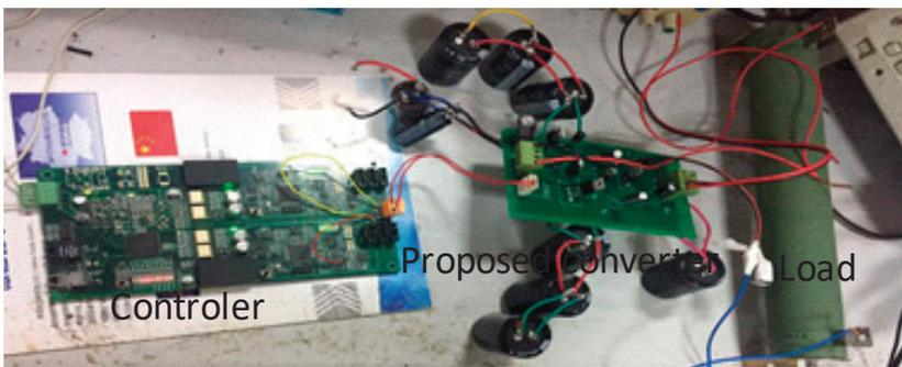
Figure 10. The prototype of the proposed converter.
