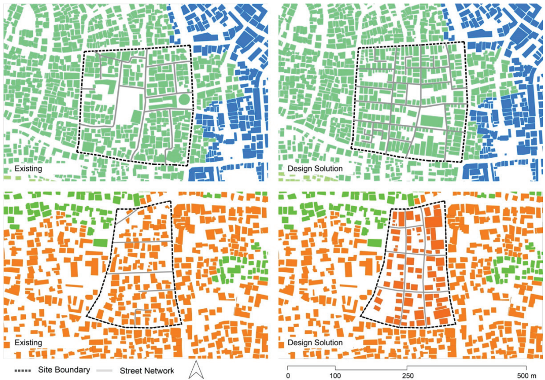
Figure 8. Two sample sites with existing fabrics ( top left, bottom left ) and two figure-ground design demonstrations ( top right, bottom right ) proposed by the same designer, in compliance with their morphometric profiles, UT7 and UT18, respectively.
