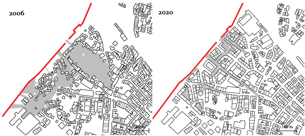
Figure 13. Visibility analysis of historical land walls (red) by creating isovist geometries in the Sulukule neighbourhood, generated on the isovist platform [28] by the Author.
