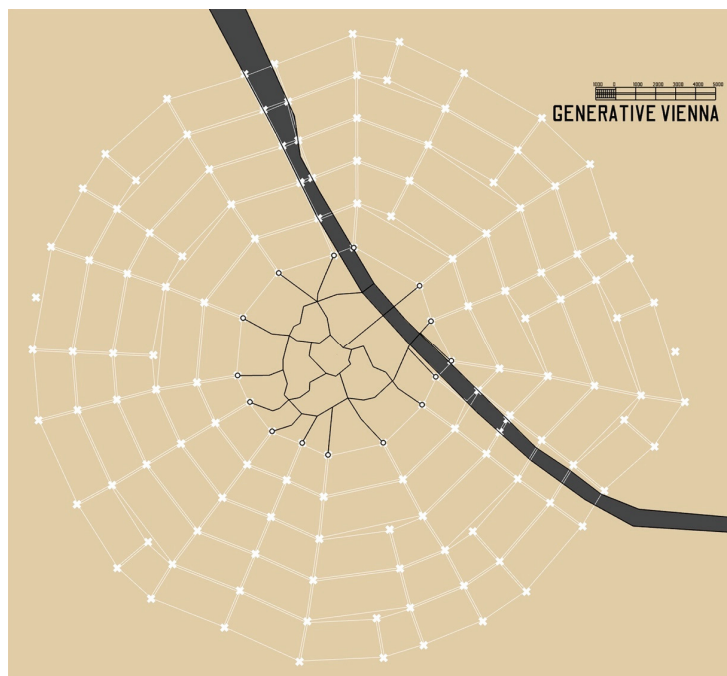
Figure 10. The generated district system using the input seen in Figure 8. Each ring of districts is generated by the same algorithm. Source: Author's work.
