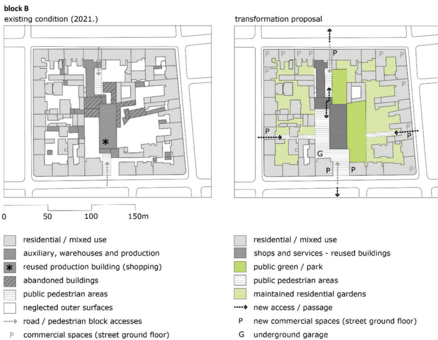
Figure 11. Transformation model of a block into a shopping and service center (example block B).
