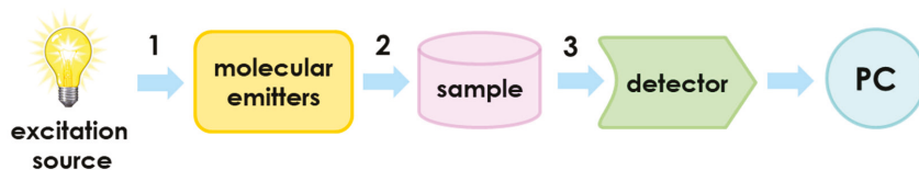
Figure 2. Block diagram of the experimental setup, where 1—exciting light; 2—emitted light; 3—transmitted light.
