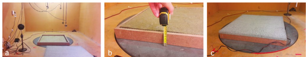
Figure 4. (a) 30 mm and (b) 50 mm rock wool filling 50 mm air gap. (c) Sample D of 20 mm over one of the two conditions.
