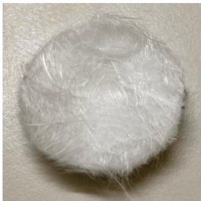
Figure 1. 10 mm diameter of fiberglass blanket samples cut for fitting into the impedance tube.
