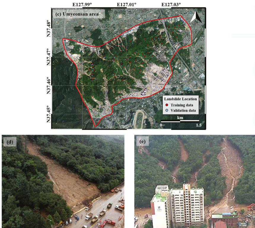
Figure 2. Data of landslide occurrence locations from aerial photographs: (a) before landslides in 2011; (b) after landslides in 2011; (c) training and validation data; (d) damage situation in Southern Circular Road [40]; (e) Gyungnam apartment buildings in Seocho-gu [41].
