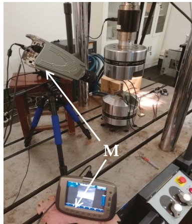
Figure 5. Tensile tests setup-Microscopy System of KEYENCE(M).
