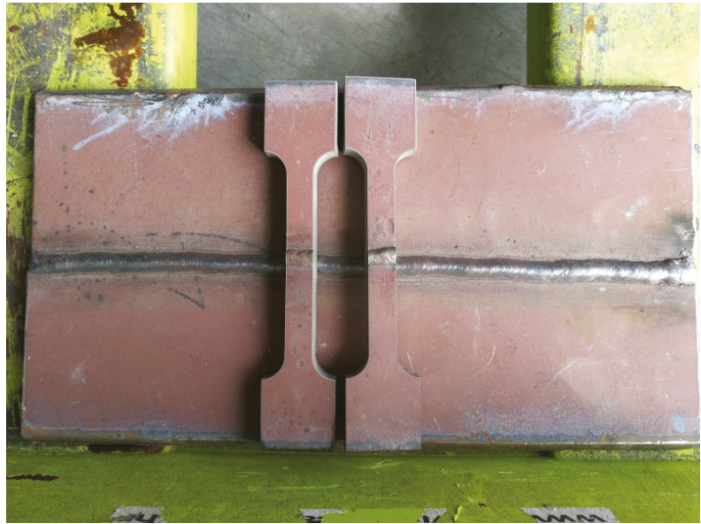
Figure 1. Welded blanks with cut out specimens.
