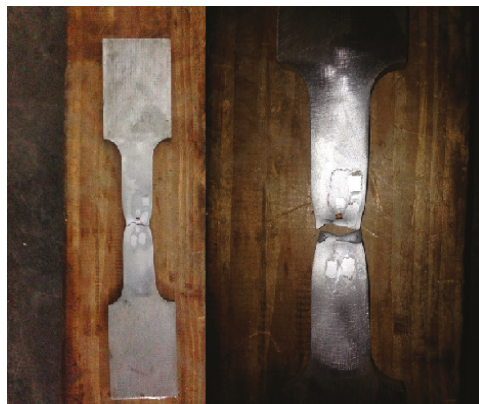
Figure 2. The fractured specimen after the tensile test.
