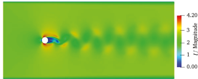
Figure 2. Velocity distribution of flow around a cylinder.
