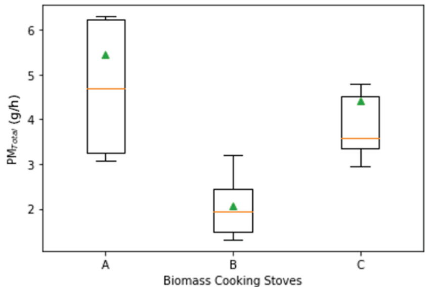
Figure 13. Total emission distribution of particulate matter in each stove.
