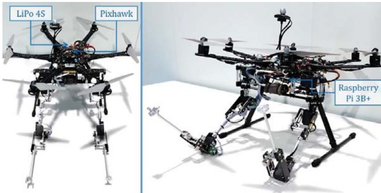
Figure 3. Dual arm aerial manipulation robot.
