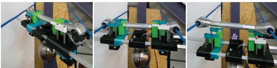
Figure 4. End effector for electrical spacers installation.
