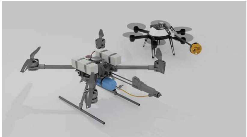
Figure 1. Two aerial robots working together to attach sensors to different parts of a bridge and similar grade separation infrastructure. The one on the left is used to spray the resin onto the surface, while the aerial robot on the right maintains contact to the surface with the sensor attached to its end-effector.
