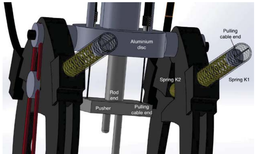
Figure 4. Detailed view of the attachment of the clamps to the linear actuator.
