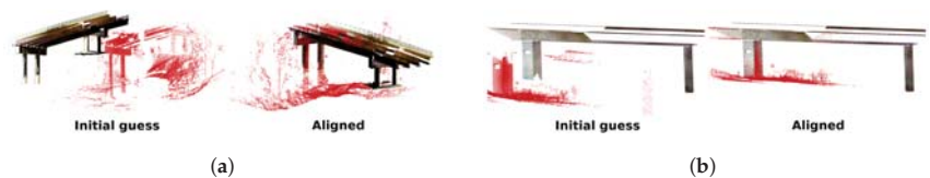
Figure 11. Global localization examples at take-off. Red points are the LIDAR reading. (a) Algodonales, (b) Álora.
