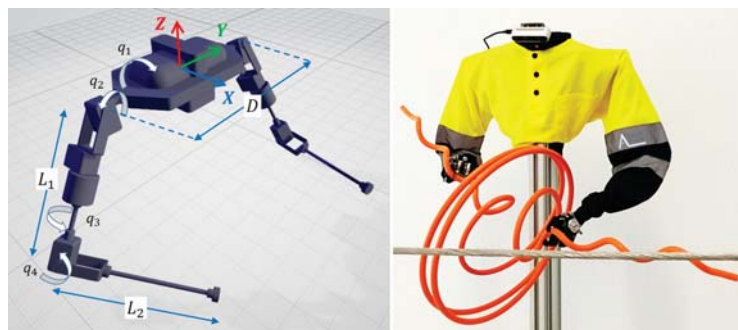
Figure 6. Kinematic model of the LiCAS A1 representing the joint angles and link lengths (left) and manipulation of helical bird diverter with LiCAS A1 anthropomorphic dual arm (right).
