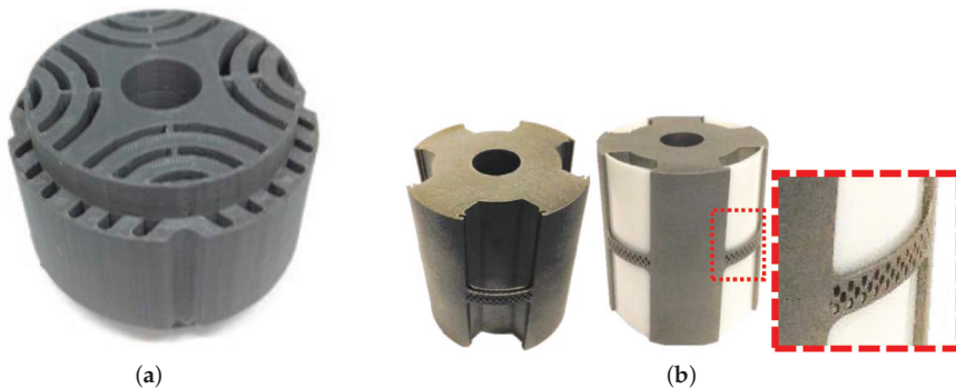
Figure 1. Additive manufactured rotor cores. These structures were fabricated without molding and tooling. (a) Printed rotor core for a synchronous reluctance machine [21]; (b) Printed rotor core for a switched reluctance machine [22].
