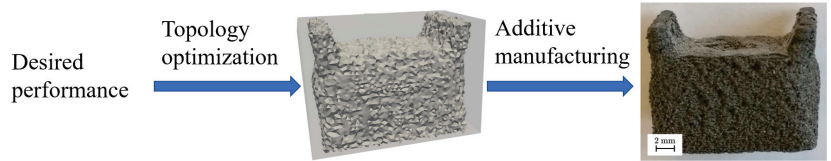
Figure 17. Topology optimized magnet. The design is then additively manufactured via fused deposition modeling. Figure is modified from [71].
