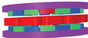
Figure 7. The three-dimensional (3D)-FEA model of the machine when one magnet is partially demagnetized.
