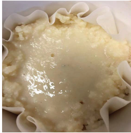
Figure 5. The precipitate in a difficult state of filtration at pH 4.0 after adding \text{Na}_2\text{CO}_3 .
