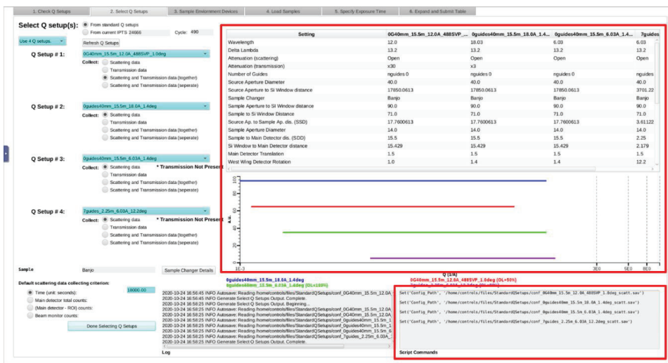
Figure 8. Friendly table view and visualization of Q-ranges (highlighted by the upper red rectangle box), scripting snippets generating with Q-range configurations selected (lower red box). The example shows up to four Q setups at the same time.
