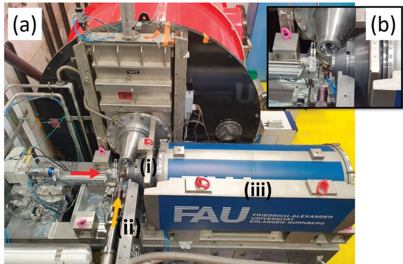
Figure 1. (a) Three lead shielding walls: (i) a cone of lead-based material, (ii) lead wall along the final part of the neutron collimation line, and (iii) a lead wall (2 tons) along the vacuum chamber of the X-ray detector. The shielding walls can be easily craned and then firmly attached to the metal chassis of the SAXS setup. Red and yellow arrows indicate the directions of the X-ray and neutron beams, respectively. The unshielded SAXS instrument (detector) represents a configuration where the lead shielding walls i, ii, and iii are not implemented during SAXS operation. A double-energy threshold X-ray detector was placed inside the vacuum tube, replacing the previously employed single-energy threshold detector. (b) A zoomed-in detail of the sample environment of the SAXS/SANS instrument, displaying a sample at an angle of 45° relative to both of the orthogonal neutron and X-ray beams.
