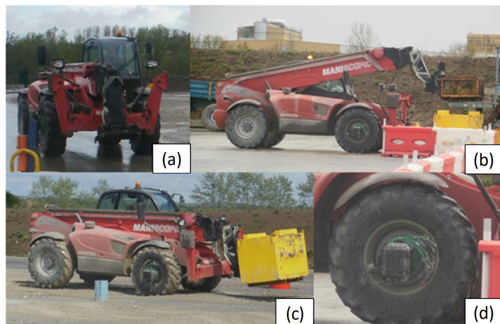
Figure 2. Different load conditions applied to the machine: (a) on-road case; (b) load placement case; (c) off-road case; (d) strain gauges and data system applied to the wheel to acquire and register the strain time-histories.
