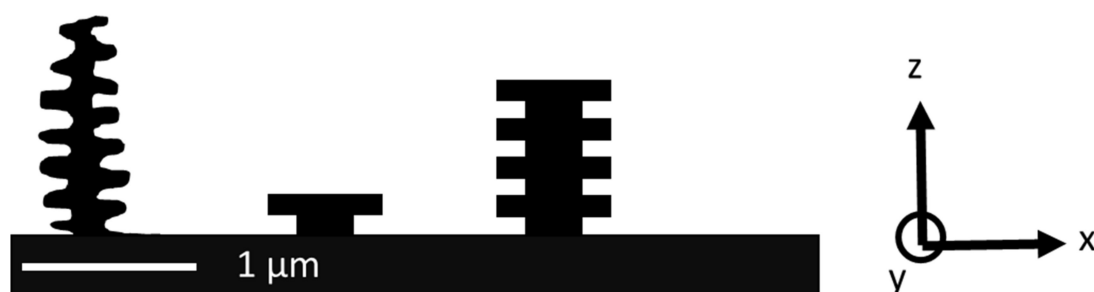
Figure 1. Left: sketch of the cross-section of the nanostructures responsible for the metallic-blue color of the Morpho butterfly. The sketch was created after images found, e.g., in [12,33]. Center and right: model structures used in this work. We started with a single layer “T-structure” and continued to work with the more complex “tree-structure”.
