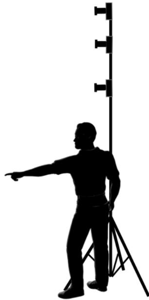
**Figure 2.** Diagram of the vertical rig with three cameras. Image by the authors.
