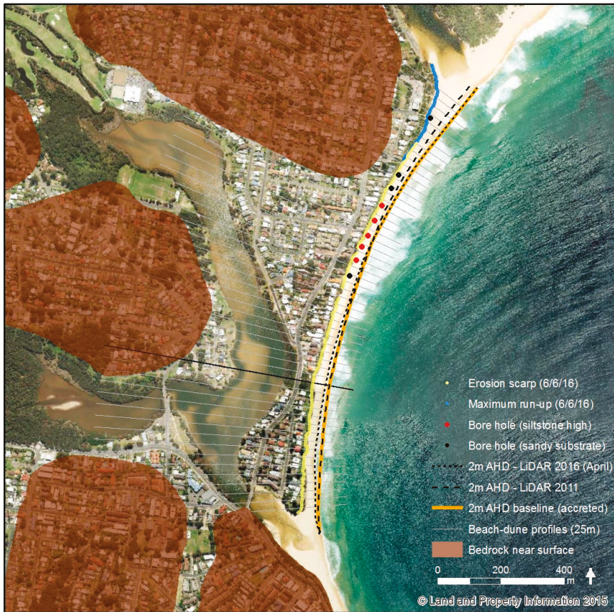
Figure 10. Wamberal Beach, which is the central sector of the Terrigal-Wamberal sub-compartment (Figure 3B), showing the distribution of 25-m alongshore-spaced beach-dune profiles that were used to calculate fluctuating shoreline change. The black profile spans the narrow point of the barrier. Beach berm positions (2 m AHD elevation contour) based on airborne LiDAR surveys carried out in 2011 and 2016 (April) are shown with the hybrid (orange) baseline representing a fully accreted beach. Bore holes sampled by Hudson [104] are also shown, indicating where a buried siltstone deposit approaches the beach face (red). The base of the erosion escarpment (yellow) and the limit of wave run-up (blue) from the June 2016 storm were mapped using RTK-GNSS immediately after the storm.
