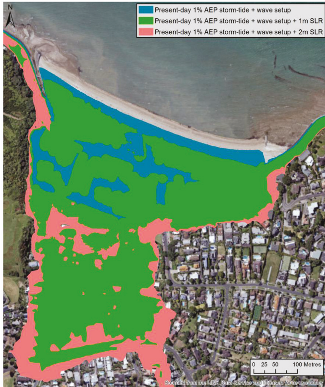
Figure 4. Coastal-storm flood mapping example at Mission Bay, Auckland. Aerial photograph of Mission Bay with present-day 1% AEP storm-tide plus wave setup elevation superimposed (blue shading), plus 1 m SLR (green shading), and plus 2 m SLR (pink shading). After: (50 @Engineers Australia, 2015).
