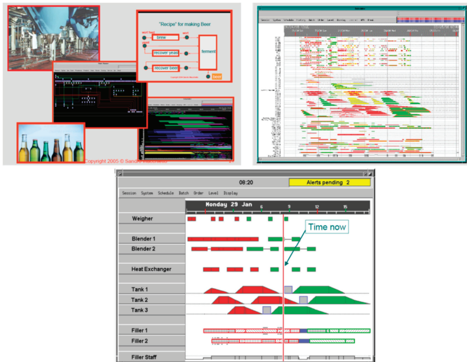
Figure 1. Top left: 14 day schedule of beer production (140 process units, 26 recipe families). Top right: 5 day production schedule of chilled desserts for northern Europe (35 product families, daily changes) as of 4:00 a.m. on a Saturday morning. Bottom: Online rescheduling every minute; the red vertical line separates the historical schedule (as actually happened) from the predicted one (adapted from [23]).
