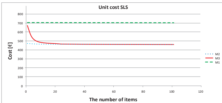
Figure 11. Dependence of the rotor production costs on the number of prototypes for SLS technology.
