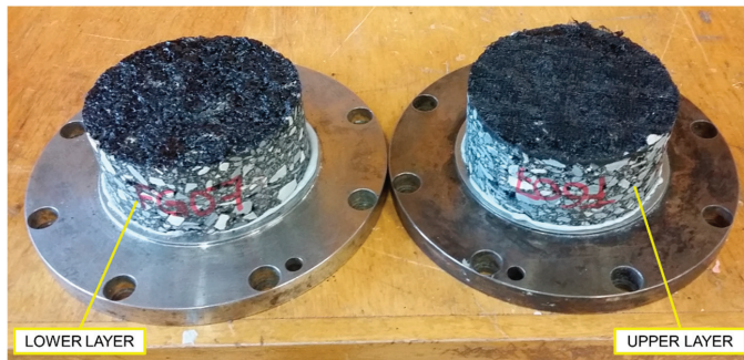
Figure 11. Failure mechanism of FG reinforced specimens at the end of shear-torque fatigue test.
