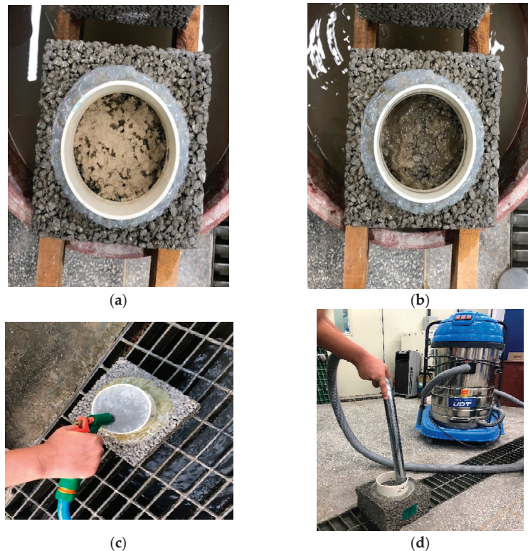
Figure 7. Void clogging test. (a) application of the blocking material; (b) after water penetration; (c) high pressure watering; (d) vacuum cleaning.
