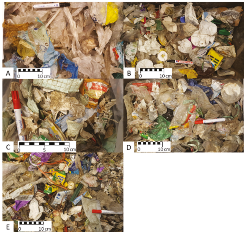
Figure 11. Exemplary photos of plastic types sorted with NIR: PE—(A); PP—(B); PET—(C); PS—(D); and others—(E) [45].
