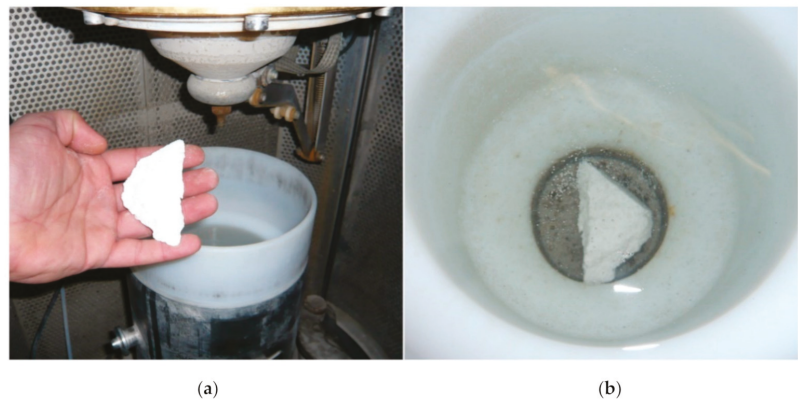
Figure 4. Fragmentation of the RefMat-2 sample. Placing the sample in the process vessel (a) and underwater sample in the process vessel (b).
