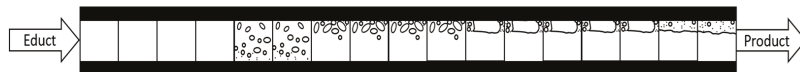
Figure 4. Sketch of the discrete calculation of the tubular reactor with a finite-element method.
