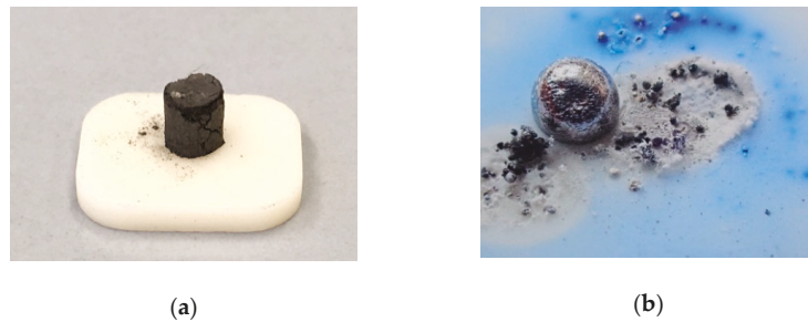
Figure 4. (a) NMC_C sample before and (b) after heating to 1600 °C in the heating microscope.
