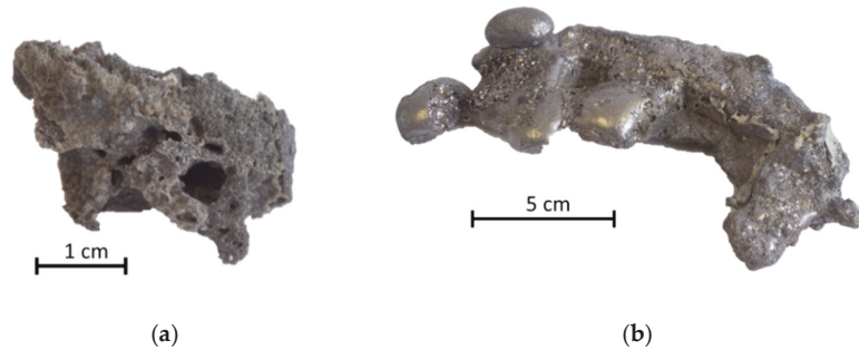
Figure 9. Obtained slag (a) and metal sample (b) from the experiment IM_NMC_C.
