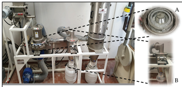
Figure 2. Micronizer pilot plant improved through the addition of a grinding chamber including a hammer crusher impeller (A) and a decanting collector (B).
