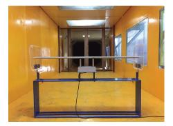
Figure 10. Aerodynamic admittance function identification test.
