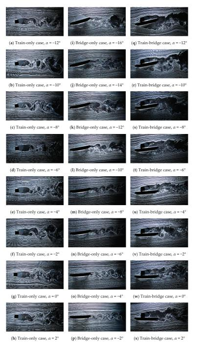
**Figure 3.** Instantaneous flow patterns: (**a**–**h**) Train-only case at  $\alpha = -12^{\circ} \sim 2^{\circ}$ , (**i**–**p**) Bridge-only case at  $\alpha = -12^{\circ} \sim 2^{\circ}$ , and (**q**–**x**) Train-bridge case at  $\alpha = -16^{\circ} \sim -2^{\circ}$ .
