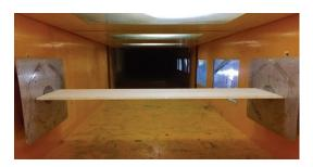
Figure 8. Three-component force test of sectional model.
