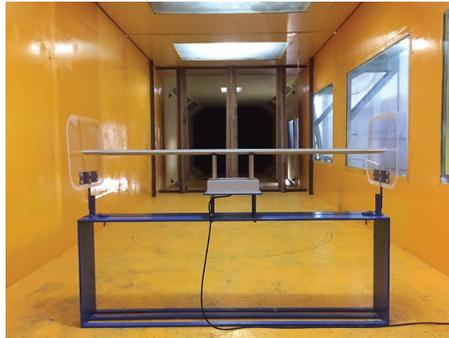
**Figure 10.** Aerodynamic admittance function identification test.
