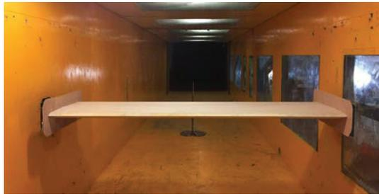
**Figure 9.** Aerodynamic derivative identification test.
