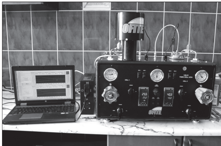
Figure 6. Apparatus for testing the build-up of static structural strength in slurry—two-chamber UCA SGSM Ofite model 120-53.
