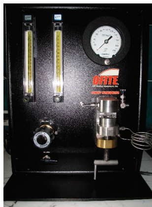
Figure 6. OFITE gas permeability meter.
