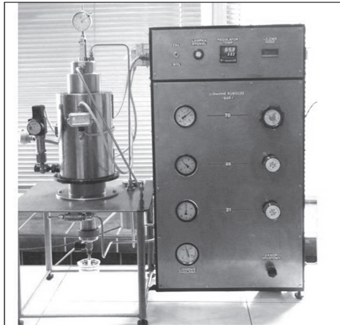
Figure 4. Apparatus for testing gas migration during slurry bonding—hydraulic press (OGI-NRI design).
