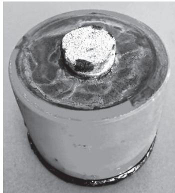
Figure 4. Sample prepared for adhesion tests.
