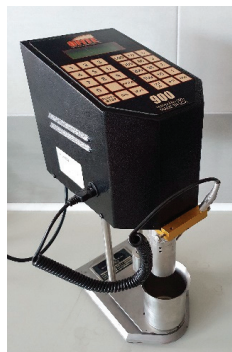
Figure 2. Fann model 900 rotary viscometer.
