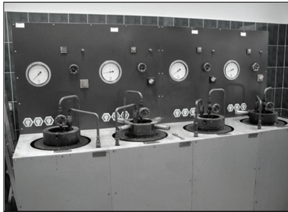
Figure 12. Autoclaves for storing samples of cement slurries.
