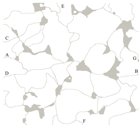
Figure 5. The pore structure of the core. A–G represent the inlet or outlet at different cases.
