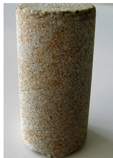
Figure 2. A core cut from a sandstone sample [27].
