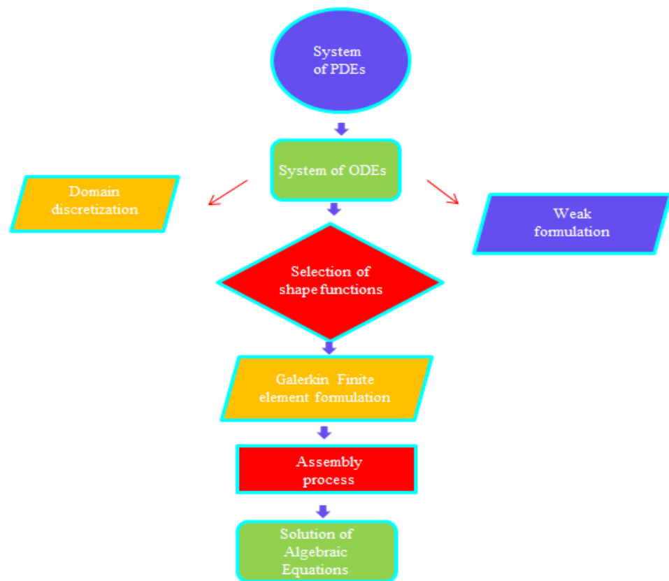
Figure 3. Flow chart regarding the finite element scheme.
