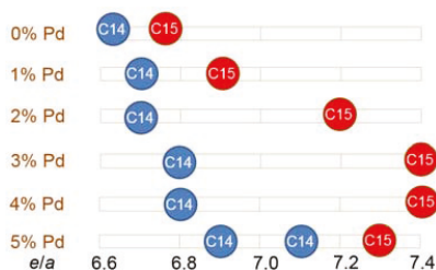
Figure 9. Plots of the e/a values for the C14 and C15 phases. A shift in the C14/C15 threshold to a higher e/a value with increasing Pd-content in design is observed.
