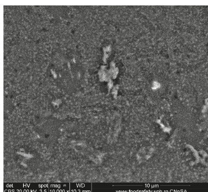
Figure 10. SEM image of 1.1%rGO-SiO 2 /glass.
