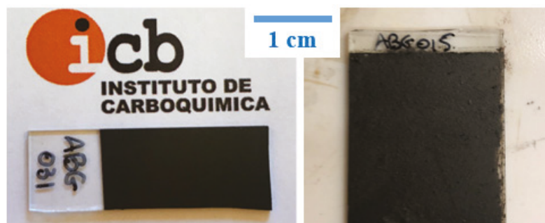
Figure 4. Photographs of films made from low-viscosity inks (left) and high-viscosity pastes (right) on glass substrates.
