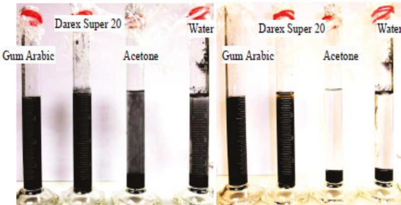
Figure 4. Stability test for graphite suspension in various dispersant of liquid at 5 min (left) and 30 min (right). Reproduced with permission from [79], ME. Thesis, National University of Singapore, 2012.
