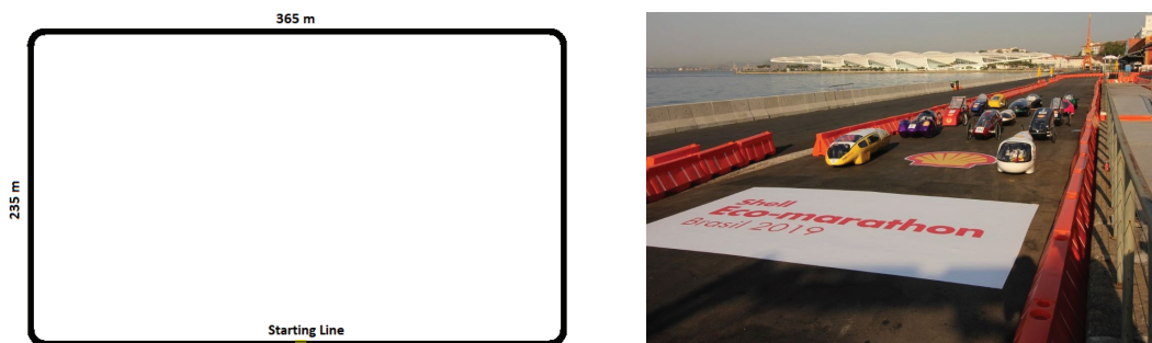
Figure 1. Circuit diagram and image of the Brazilian start line for the Shell Eco-marathon competition (5 m wide rectangular circuit with 90° curves with an 8 m radius).
