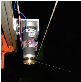
Figure 7. Electric servomotor and its worm damping the mooring line.
