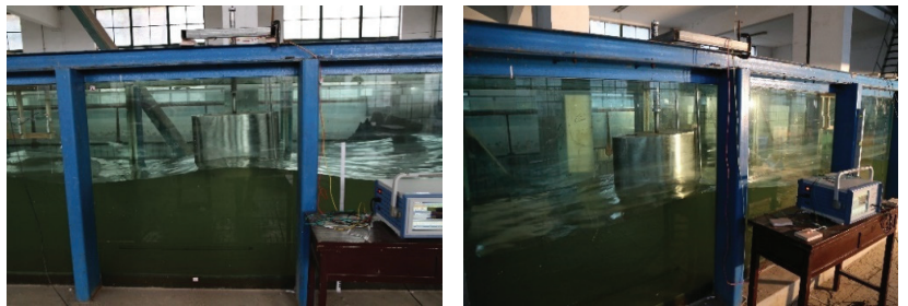
Figure 5. Installation of WEC experimental device in flume.
