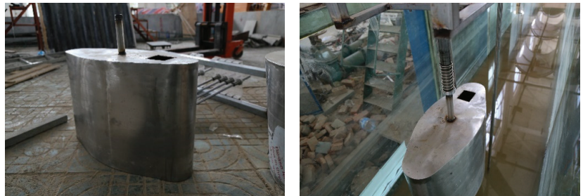
Figure 3. The elliptical cylinder of oscillating buoy.
