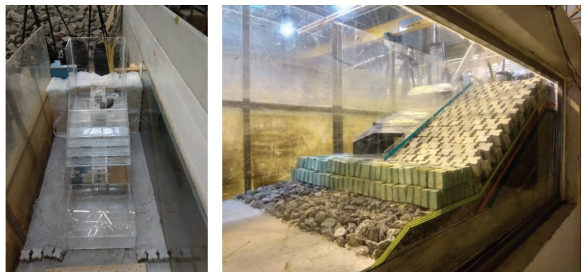
Figure 4. Frontal view of the OWEC–OWC model (left) and perspective of the physical model setup for the extreme wave tests (right).
