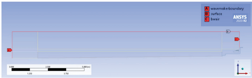
Figure 7. Wavemaker, top surface and air boundary of the computational domain.
