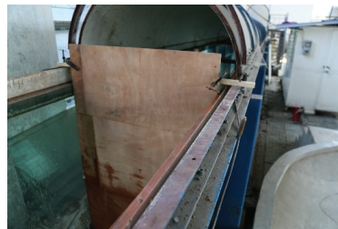
Figure 9. Wooden rigid vertical baffle (inducing fully standing waves) installed in flume.
