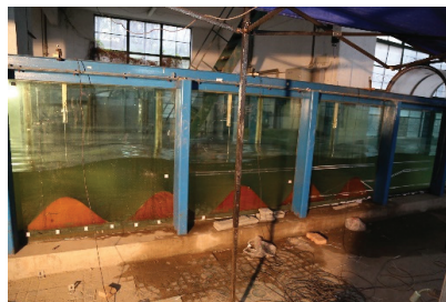
Figure 6. Five fixed continuous sinusoidal wavy bottoms installed in flume.
