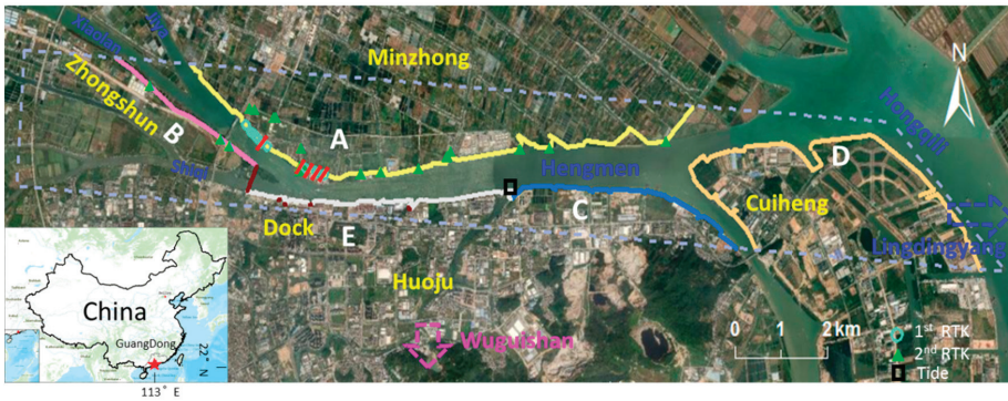
Figure 1. The airborne LiDAR surveyed areas (gray dashed line) in the Hengmen waterway of the Pearl River Delta, Zhongshan, GuangDong Province, China. The triangles, circles and red lines are the locations of in situ elevation measurement using GPS-RTK. The black square is the site of the Hengmen tidal station. The surveyed levees are divided into five segments from A to E.
