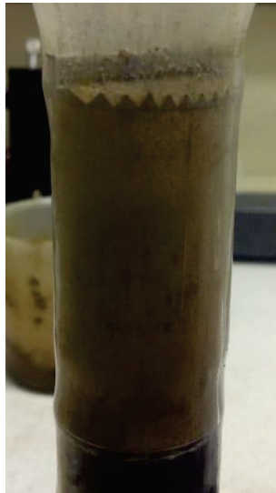
Figure 8. Bulk model with screen filter disk installed.
