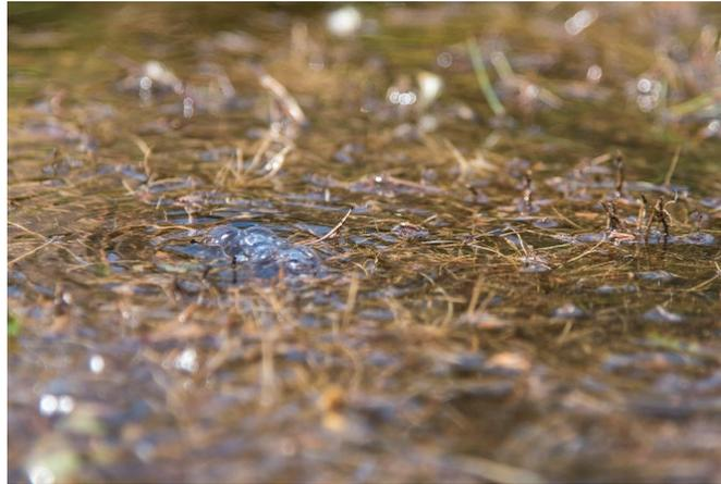
**Figure 12.** Significant bubbles during the filling process indicating (preferential) flow during the drought period: air-filled pores are filled with water forcing out the trapped air.
