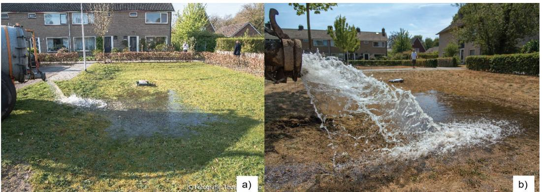
**Figure 6.** The full-scale infiltration test with a tank truck executed repetitively for monitoring the hydraulic behaviour of swales in Dalfsen—(a) under regular conditions in 2017, (b) Same monitoring after 7 weeks of drought in 2018.
