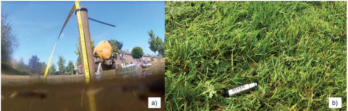
**Figure 7.** The methods for monitoring the water height in the swales during the infiltration tests were (a) hand measurements on a measuring tape and underwater video camera, continuous time-lapse photography (b) and pressure transducer loggers.
