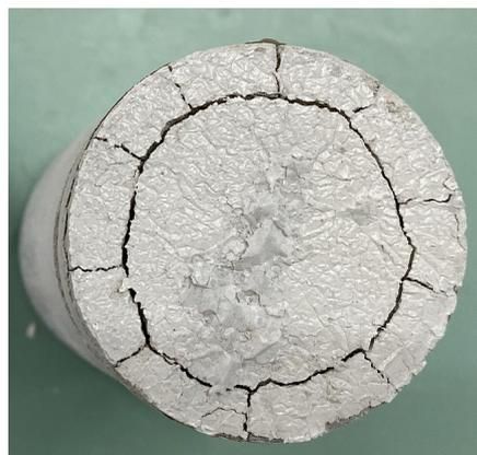
**Figure 4.** Contraction cracking caused by high water content.
